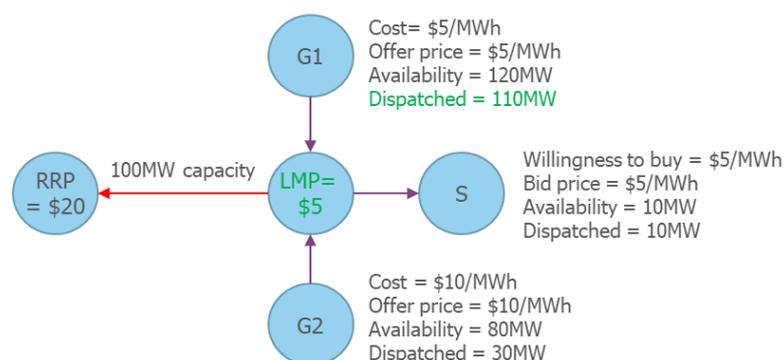
Both generator 1 and 2 are solar generators, and the dispatch interval is in the middle of the day. As a result, both generators are capable of generating a combined output of 200MW, absent of transmission congestion. The introduction of a storage unit, S, means that 10MW more generation is dispatched, all of which is from generator 1 as it is the cheapest and still has sufficient capacity. Less renewable generation is spilt.
